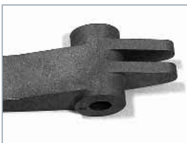
Fe hinge: 225kV; 3 mA
